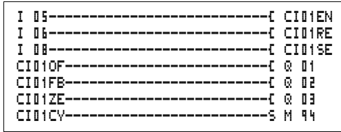
Figure 106: MFD-Titan circuit diagram with high-speed incremental encoder counter
