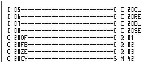
Figure 100: MFD-Titan circuit diagram with counter relay
