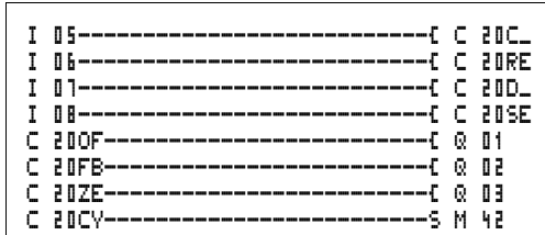
Figure 71: easy800 circuit diagram with counter relay
