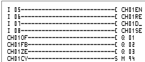
Figure 75: easy800 circuit diagram with high-speed counter
